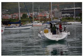
▶ Preparation is a key moment of the mooring manoeuvre. When approaching the berth, the lines must already be coiled and ready to tossed, and the fenders must be in place
